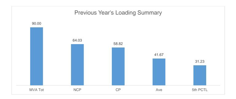
The Non-coincident Peak Demand is 64.03 MW, which is around 71.14% of the total substation capacity of 90 MVA at a power factor of 0.97. The load factor or the ratio between the Average Load of 41.67 MW and the Non-coincident Peak Demand is 65.08%. A safe estimate of the true minimum load is the fifth percentile load of 31.23 MW which is 48.77% of the Non-coincident Peak Demand.
