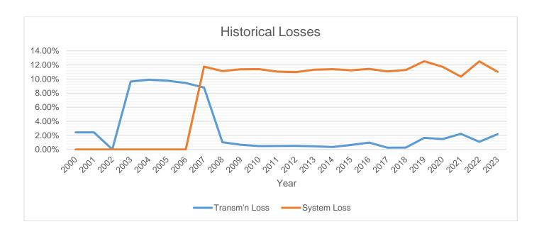
Historically, Transmission Loss ranged from 0% to 10% while System Loss ranged from 10% to 13%. Transmission Loss peaked at 9.90% on year 2004 due to the fact that the power transformers were inefficient during that time. System Loss peaked at 12.53% on year 2019 because of circuit configurations and optimization of maximum loading capacities of adjacent feeders that needs to be addressed.
